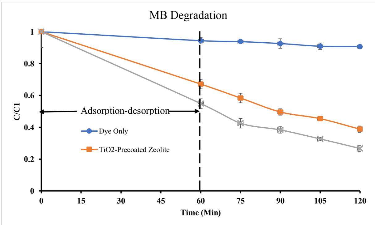
Figure 6: Time-dependent degradation profiles for all zeolite samples and control experiment (Dye Only).
