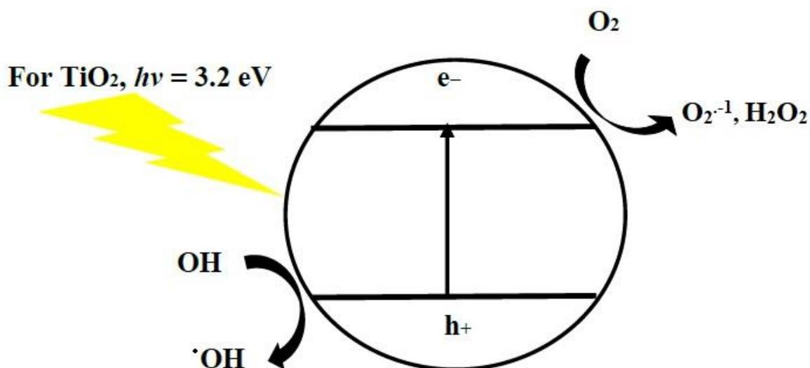
Figure 4: Schematic representation of the mechanism of photocatalysis on titanium dioxide particles.
