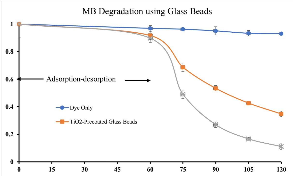
Figure 5: Time-dependent degradation profiles for all glass bead samples and control experiment (Dye Only)
