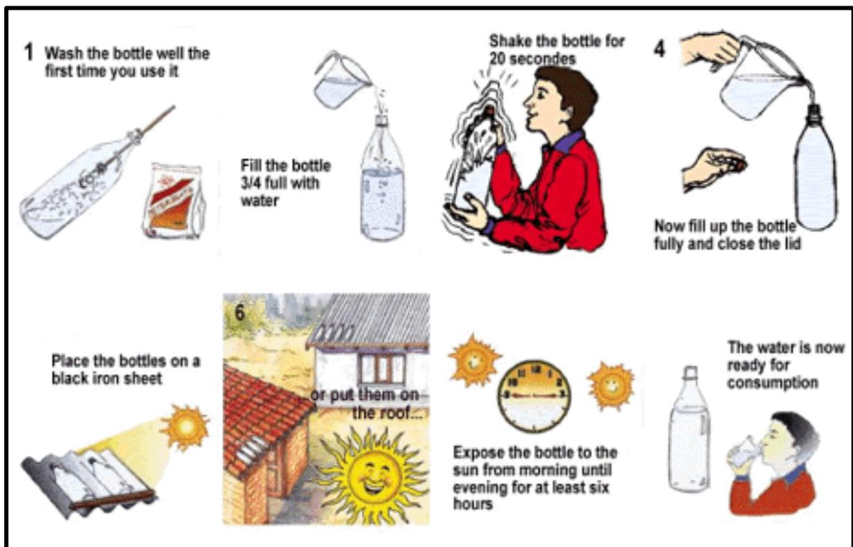
Figure 1: Pictorial representation of the stages involved with the SODIS method. 24
